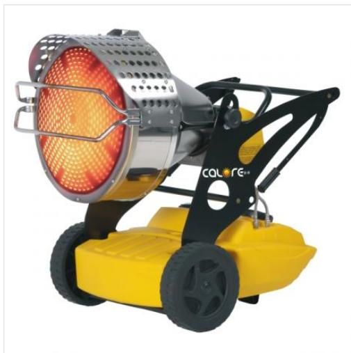
**CARACTERISTICI TEHNICE**Putere calorica ( kW ): **43**Putere cal. ( kcal/h ): **36.980**Consum carburant ( l/h ): **3.6**Capacitate rezervor ( l ): **60**Consum energie ( W ): **140**Frecventa ( Hz ): **50**Combustibil: **Motorina**Dimensiuni ( mm ): **1070x700x980**Greutate ( Kg ): **69****DESCRIERE PRODUS**
