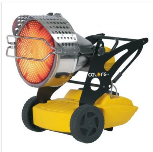
**CARACTERISTICI TEHNICE**Putere calorica ( kW ) : **29-43**Putere cal. ( kcal/h ) : **24.940-36.980**Consum carburant ( l/h ) : **2.3-3.37**Capacitate rezervor ( l ) : **60**Consum energie ( W ) : **160**Frecventa ( Hz ) : **50**Combustibil: **Motorina**Dimensiuni ( mm ) : **1070x700x980**Greutate ( Kg ) : **69****DESCRIERE PRODUS**
