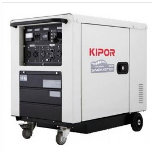
**CARACTERISTICI TEHNICE**Putere maxima ( kVA ): **5.5**Motor: **HONDA OHV**Tip motor: **KD186FGETi**Capacitate cilindrica ( cmc ): **418**Combustibil: **Benzina fara plumb**Consum combustibil ( g/kW h ): **340**Autonomie ( h ): **7**Frecventa ( Hz ): **50**Tensiune ( V ): **230**Turatie grup ( rpm ): **1700-3000**Nivel de zgomot ( db A ): **97**Numar de faze: **monofazat**Capacitate baie de ulei ( l ): **16**Dimensiuni ( mm ): **90x57x79**Greutate ( Kg ): **168****DESCRIERE PRODUS**
