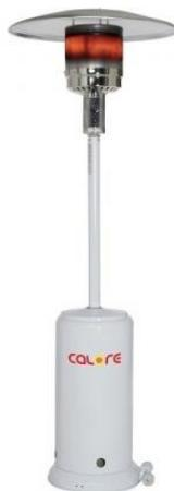
**CARACTERISTICI TEHNICE**Putere calorica ( kW ): **5-13**Put. calorica ( kcal/h ): **11.200**Combustibil: **propan / butan (butelie GPL)**Consum de gaz ( Kg/h ): **0.45-0.87**Trepte de putere: **2**Aprindere: **Manuala**Material: **Otel inoxidabil**Inaltime ( cm ): **224**Greutate ( Kg ): **20.5****DESCRIERE PRODUS**
